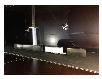
The Pressure Fluctuation Monitoring System will be installed on a container shipped on a freight train to validate wind tunnel measurements of the aerodynamic properties of the depicted model
