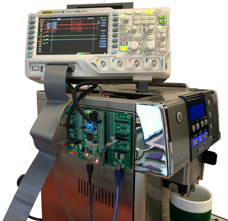
Figure 2.6: The prototype used for this thesis, using the STM32F407 evaluation board along with an breakout module for easy access of all SPI-busses, connected to the machine as well as a logic analyzer. The final board will be comprised mostly of the CPU and electrical isolation.
