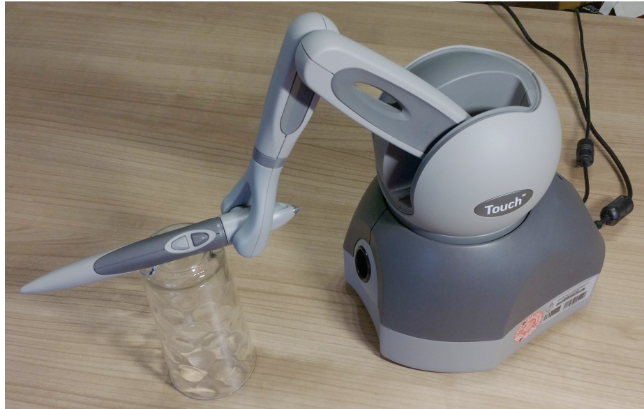
Figure 2.3: Picture of the 3D Systems Touch™ haptic device. The glass is not part of the device and is only utilized as a professional holding solution.
